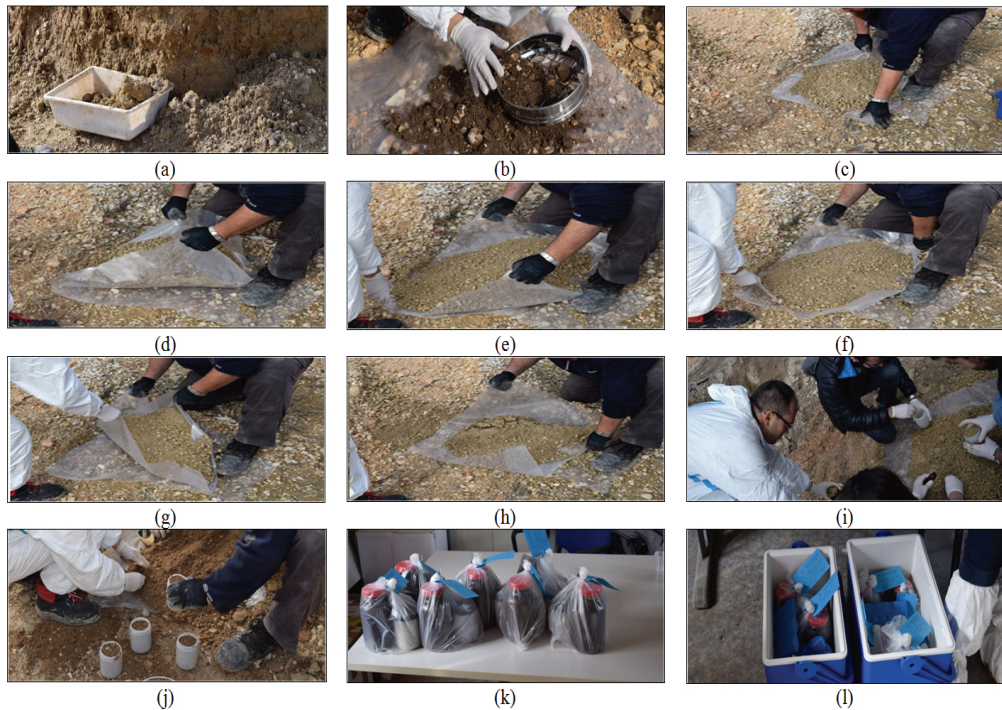
Fig. 4. Main steps of the excavation faces verification: (a) Sampling from the excavation; (b) Sieving; (c-h) “Quartering method” by mixing of soil subsamples; (i-j) Final sampling; (k) Samples of soil ready for analysis; (l) Transport to the laboratory.
