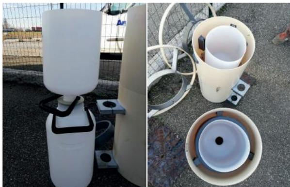
**Fig. 3** – Deposimetro in HDPE.
