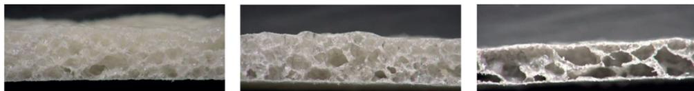
**Fig. 5** – Foamed PVC layer: Left) Reference, no recycle; Middle) 3 wt% recycle; Right) 12 wt% recycle
