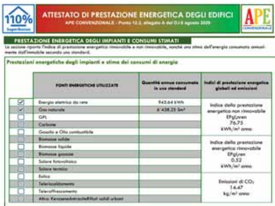
Fig. 2. Energy performance certificate (in Italian = APE) after the interventions
