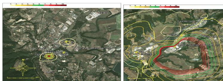
**Fig. 3.** Map of the 98<sup>th</sup> percentile of the peak odour concentration values relevant to the emissions from the industrial pole of Narni Scalo (left) and the one of Nera Montoro/ San Liberato (right), in a scale from 1 ou<sub>E</sub> m<sup>-3</sup> to 10 ou<sub>E</sub> m<sup>-3</sup>
