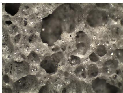
**Fig. 2.** Optical micrograph for the foam glass containing 50 wt % of glass scraps and 50 wt % cutting sludge treated at 800 °C for 30 min
