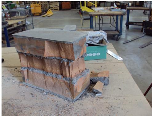
**Fig. 2.** A triplet after the compressive strength test
