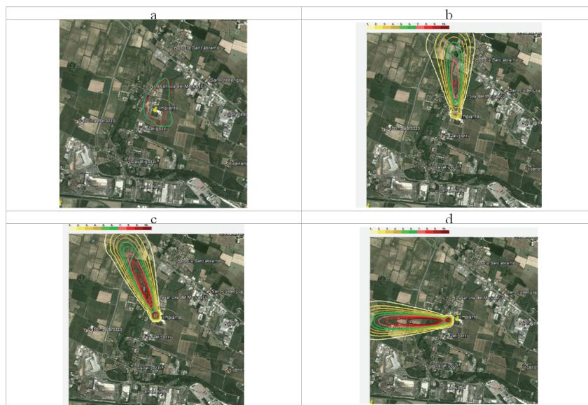
**Fig. 5.** Odour impact assessed by field inspection (a) vs. simulated by odour dispersion modelling considering different time ranges: 16-17 h (b), 17-18 h (c), 18-19 h (d)
